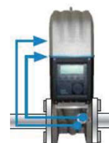
Meter with external flow conversion (p/T external)
